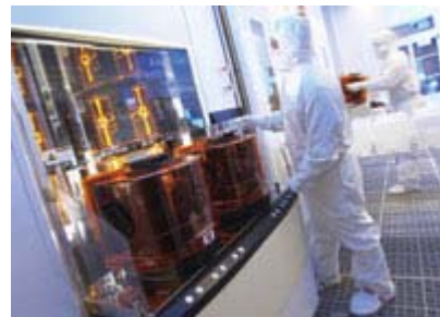
Workers for MEMC Electronic Materials strengthen silicon wafers at an annealing furnace at the company's plant in St. Peters, Mo., near St. Louis.
