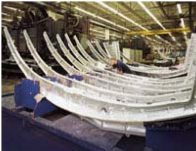
An employee of the St. Louis GKN Aerospace manufacturing facility inspects machined aluminum-alloy aircraft ribs.
